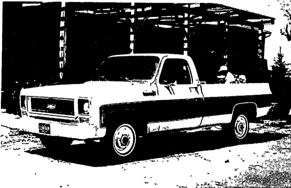
1973 CHEVROLET FLEETSIDE CHEYENNE SUPER PICKUP - Completely restyled and with extensive chassis redesign, the 1973 Chevrolet pickup line features many improvements in appearance, durability, and comfort for both commercial and personal transportation. Highlights are curved side windows, powered cab ventilation, new leaf-spring rear suspension, increased cooling capacity, a larger available engine, outside fuel tank, easier servicing, and highly styled interiors.
