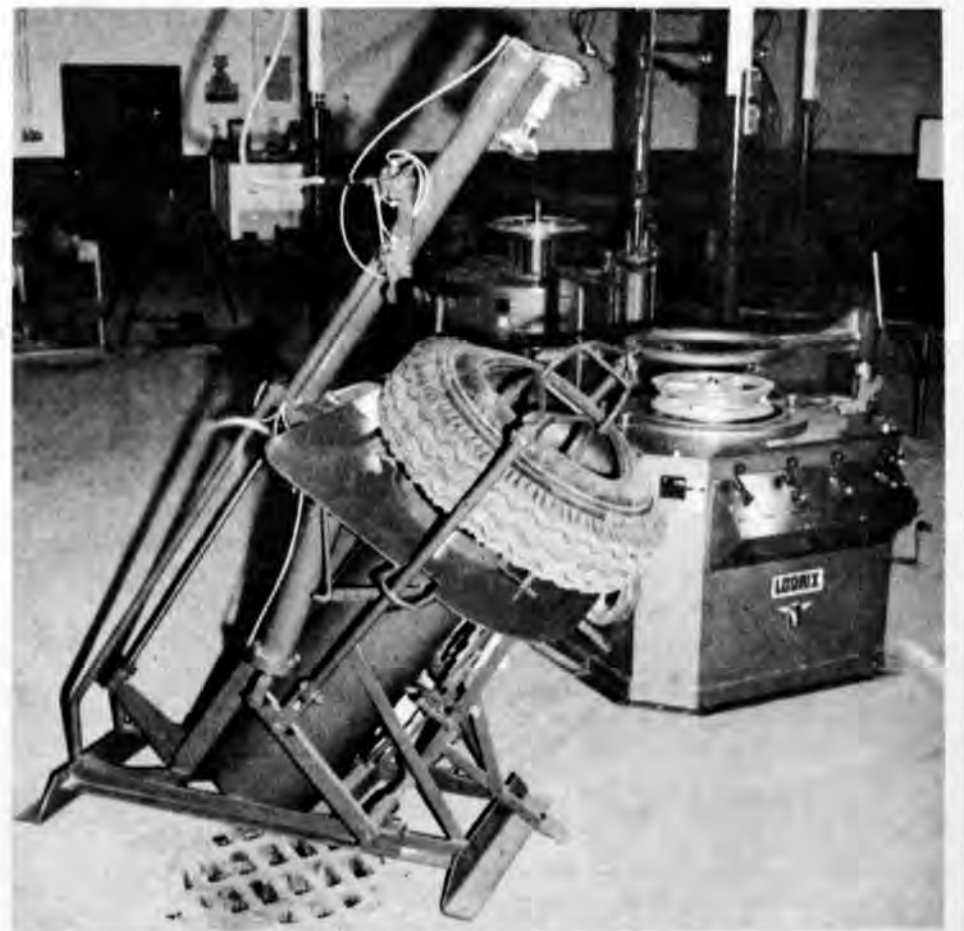
A debagger used to insert and remove the airbag from tire before and after curing. Passenger tire changer to the right rear at Jack Rhynard's Retreading Service.
