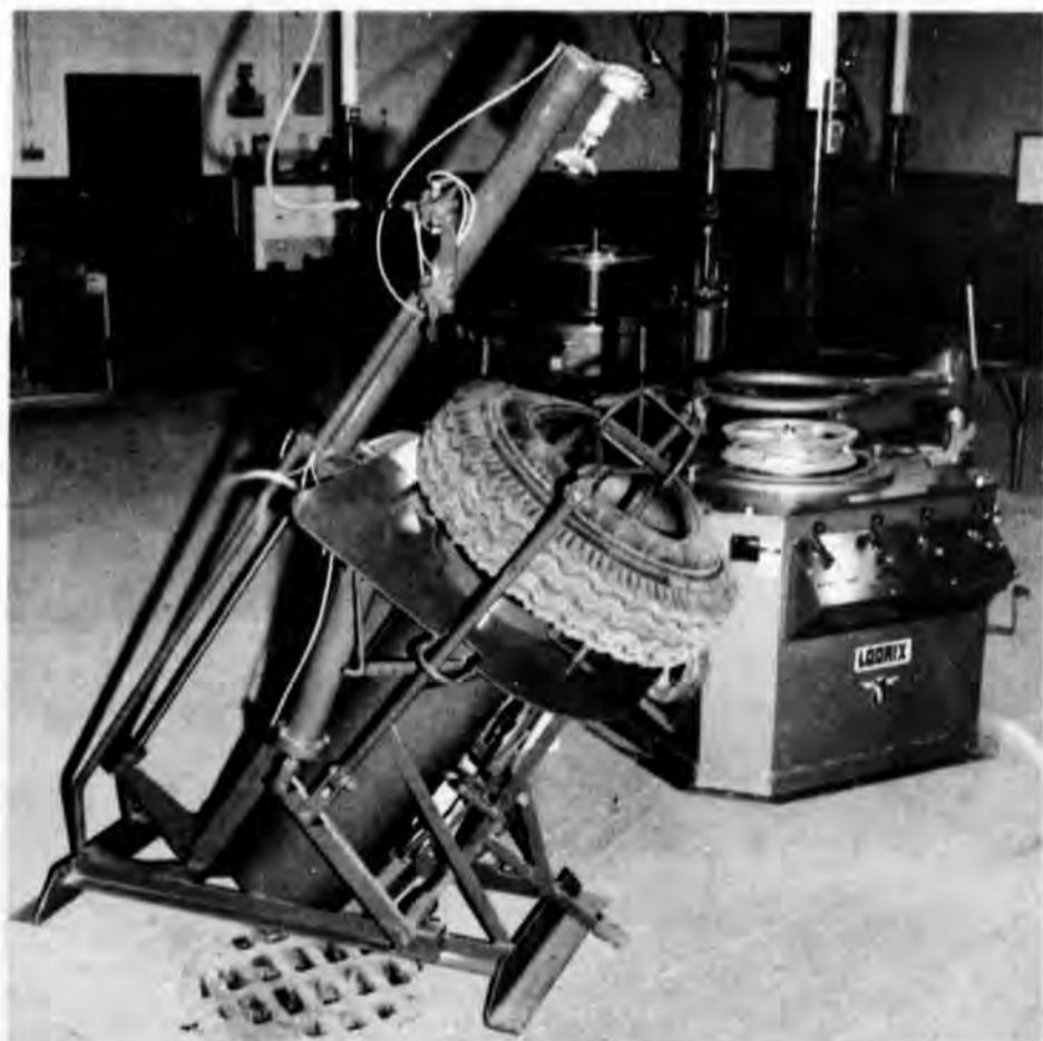
A debagger used to insert and remove the airbag from tire before and after curing. Passenger tire changer to the right rear at Jack Rhynard's Retreading Service.
