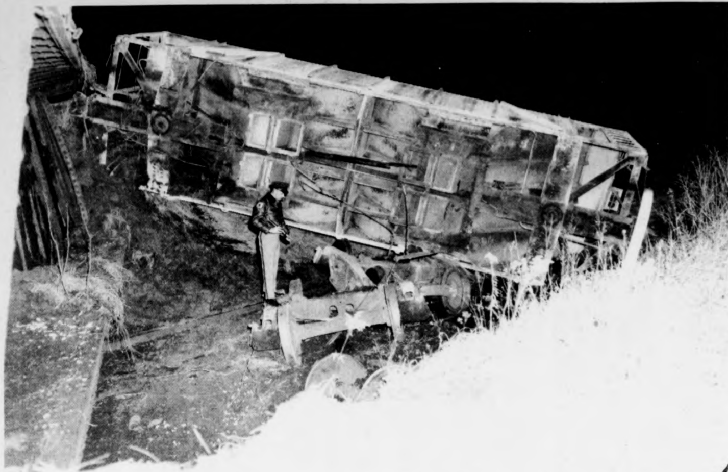
Deputy Sheriff Richard May of the Clinton County Sheriff's Department inspects wheels from one of the railroad cars derailed Sunday evening west of Laingsburg. An empty box car lies crossways on the track in the background. Huge steel girders which shifted on a flatcar are believed to have caused the derailment of 13 freight cars. No one was injured.
