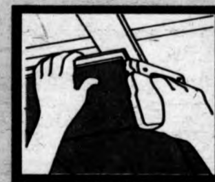
OR STAPLE tiles onto wood furring strips.
