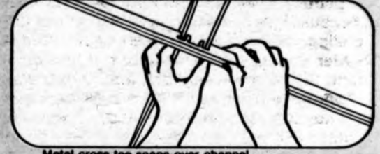
Metal cross tee snaps over channel.
