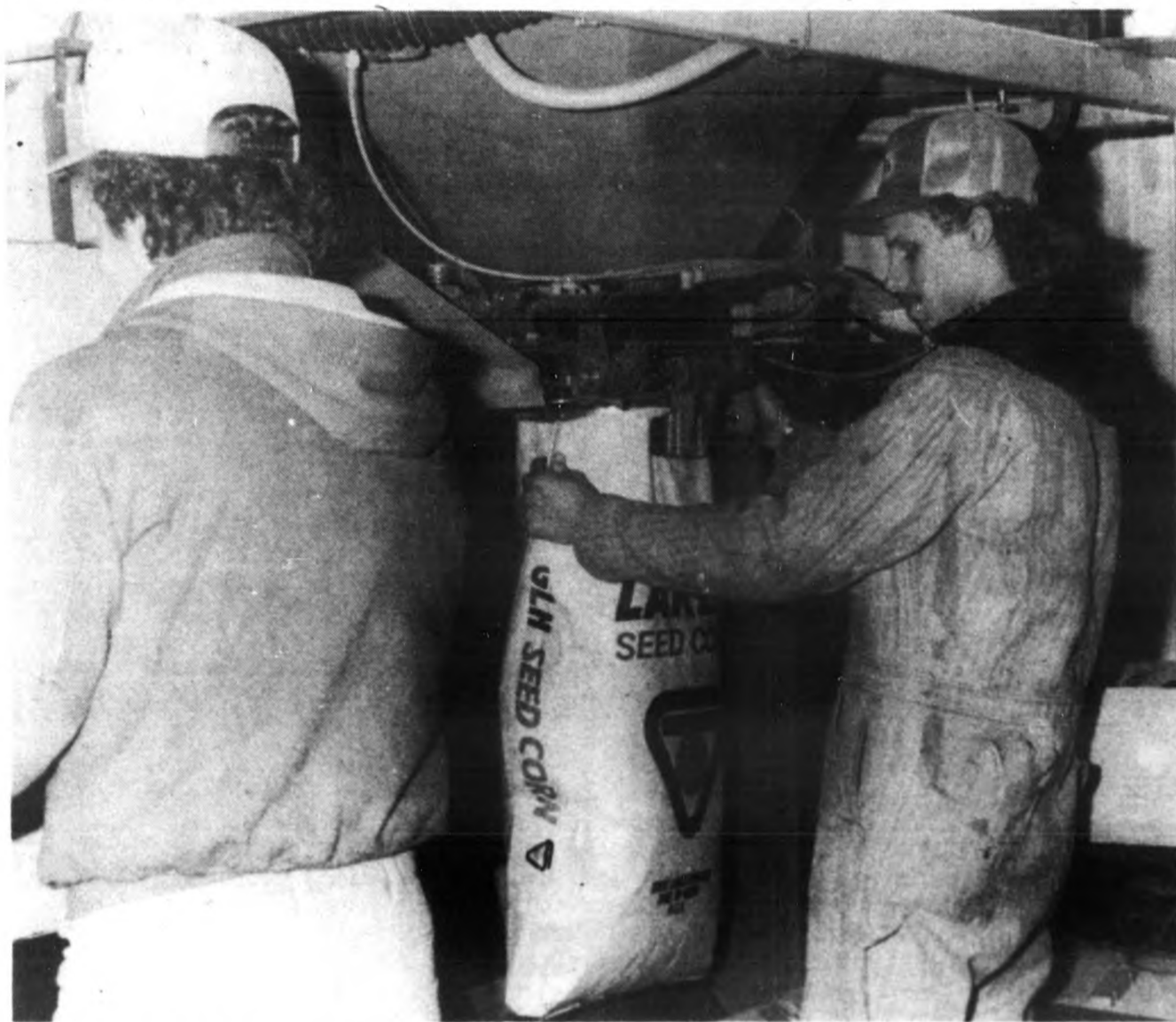
GLH WORKERS USE BAGGER-Workers at Great Lakes Hybrids operate the bagging machine. The hopper weighs out the seed and then dumps it into the bag. The weigher is calibrated to weigh within 2 ounces over the bag weight. Each bag is tagged to identify its seed classification.
