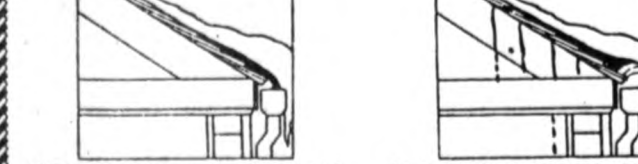
Melting snow over the heated portion of the house runs down to the roof edge it freezes and an ice dam begins to form, preventing drainage.
