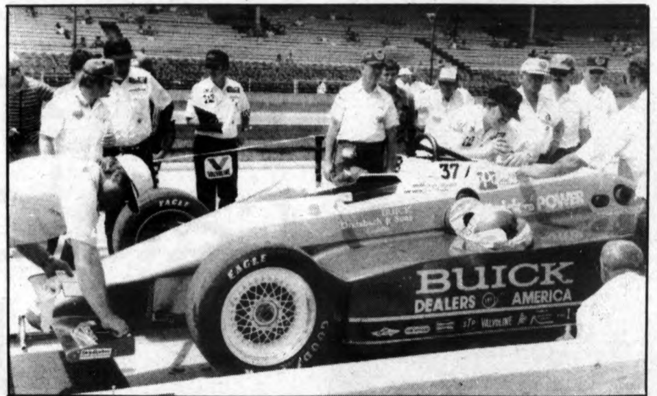
Scott Brayton, Coldwater, MI, getting a pre-qualification technical inspection on his stock block, turbo charged Buick V-6 engine car.
