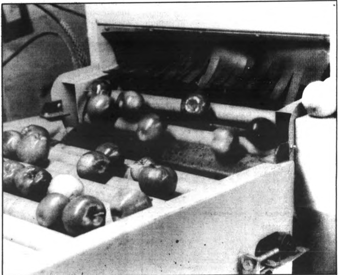
AFTER 15 MINUTES the dirty apples come out shiny clean and then head for the automatic sizer, where they are separated and bagged for purchase.
