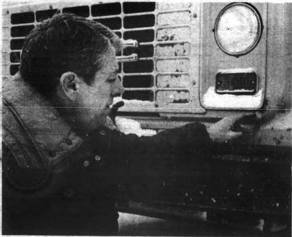
Mechanic Jack Desprez points out rust spots on a St. Johns School bus. Along with metal stress resulting from travel on rough roads with heavy loads of students, rust is a big problem for the St. Johns bus fleet, board members were told at a recent meeting. (Photo by David Olds)
