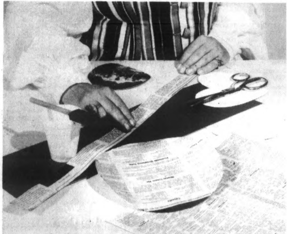
Line the posterboard side of the band box pieces with newspaper using stick glue as shown here by Greenfield Village Craftsperson Sandra Richards. Take the long piece of cardboard and form it into a roll, overlapping the edges about an inch and fasten with masking tape. Then attach the bottom.
