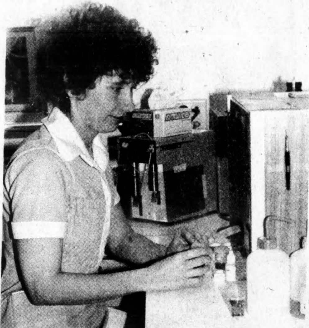
Sharon Shutes, a registered medical technologist, ASCP, works with the Hycel 700 Counter which analyzes the white and red blood cells, as well as the hemoglobin and hematocrit. (Photo by Patrice Hornak)
