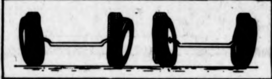
IMPROPER TOE PLACEMENT Toe-in our toe-out of wheels causes excessive tread wear.
