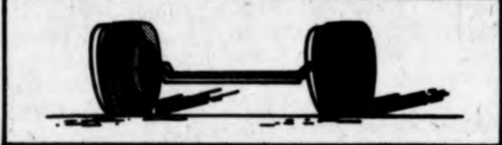
"GRABBING" BRAKES Cause the same condition as out-of-balance wheels - flat spots and bald spots.
