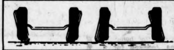
IMPROPER CAMBER (Wheels tilted in or out) causing more wear on one side of the tires.
